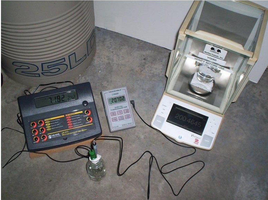
Figure1A. Photograph of the actual key experimental setup except that the 25-liter Dewar was not located near the measurements as shown but at a remote location described in the text.
